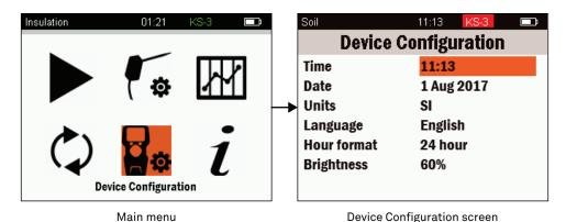
Figure 10 Device Configuration screen
