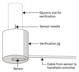
Figure 22 Verification holder for single-needle sensors
