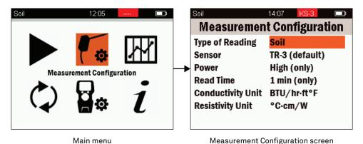
Figure 13 Measurement Configuration screen
