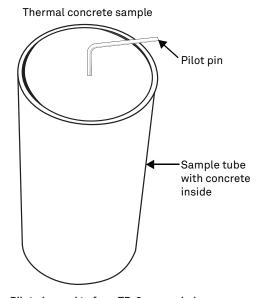
Figure 16 Pilot pin used to form TR-3 access hole
